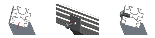
Individual profile rails are screwed together using the L-shaped profile connector and 2 M8 x 20 mm self-tapping screws.
