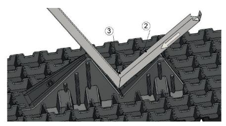
It is important to ensure that the angle bracket is correctly aligned - refer to the drawing below
