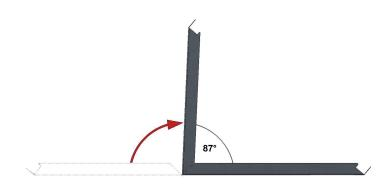
Subsequently, the angle is placed on the base plate and fastened with 4 pcs. pan-head screws 5/16" - 10 ACME. Position the pan head screws straight and centered to the internal thread of the clamping nut and tighten with the cordless screwdriver (Tightening torque  $M_A = max. 15 \text{ Nm}$ ).
