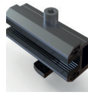
Laminat Modulklammer M_A = \text{max. } 16 \text{ Nm}
