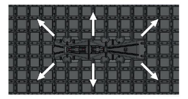
During the pouring process, make sure that no gravel / granulate gets under the base plate, this must be removed if necessary. The threaded sleeves must be kept clean.
