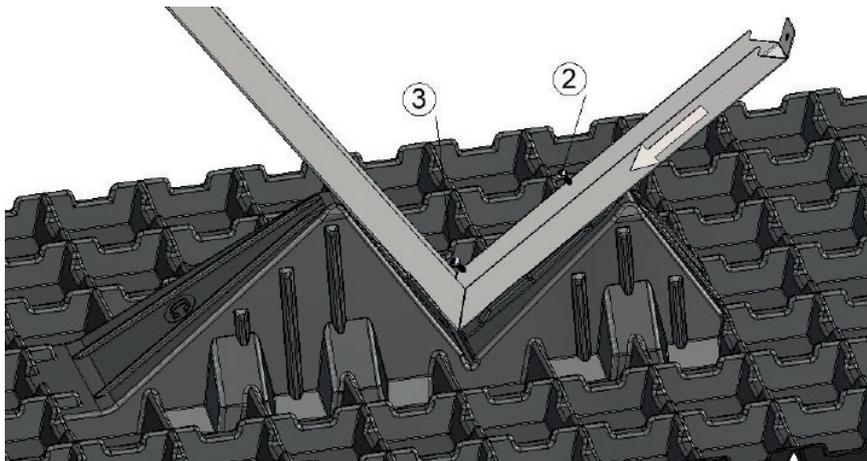
It is important to ensure that the angle bracket is correctly aligned - refer to the drawing below
