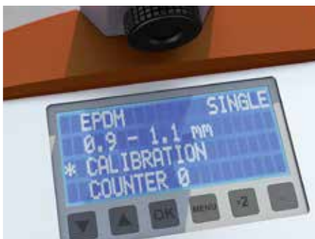
5. Switch on and calibrate the Contec.fix SFS Isoweld®3000 induction machine
