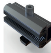
Laminat Modulklemme M_A = \text{max. } 16 \text{ Nm}
